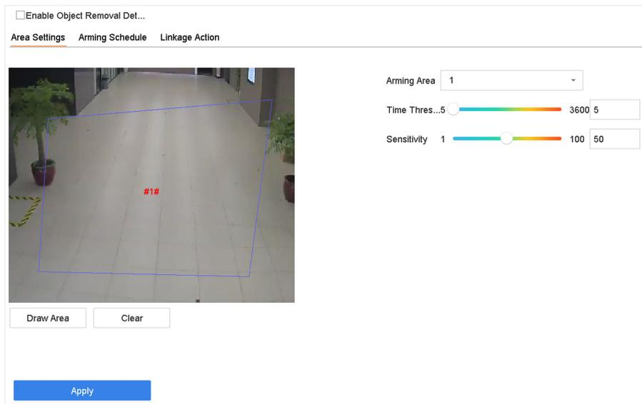
**Figure 6-16 Object Removal Detection**
