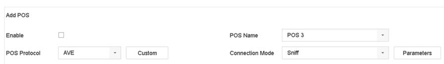
The screenshot shows a web interface for adding a POS device. It features several input fields: an 'Enable' checkbox, a 'POS Name' dropdown menu with 'POS 3' selected, a 'POS Protocol' dropdown menu with 'AVE' selected and a 'Custom' button, a 'Connection Mode' dropdown menu with 'Sniff' selected, and a 'Parameters' button.
